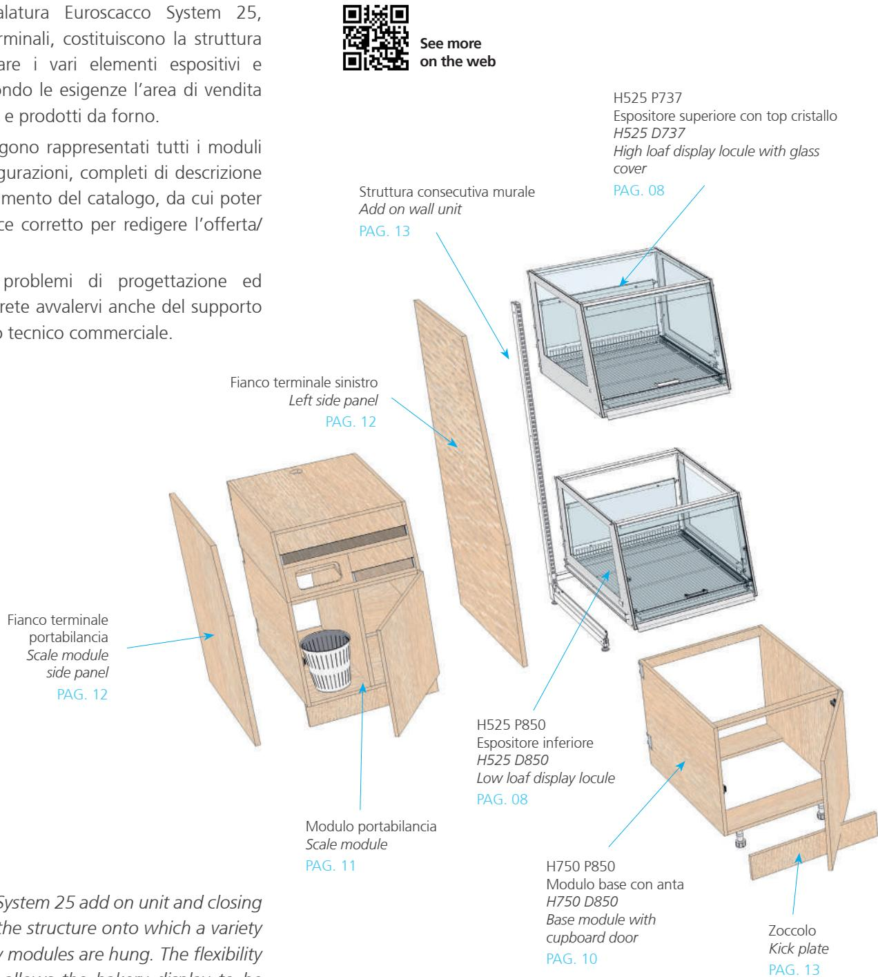
*The Euroscacco System 25 add on unit and closing frame make up the structure onto which a variety of bakery display modules are hung. The flexibility of the modules allows the bakery display to be tailored to the needs of the sales area.*
